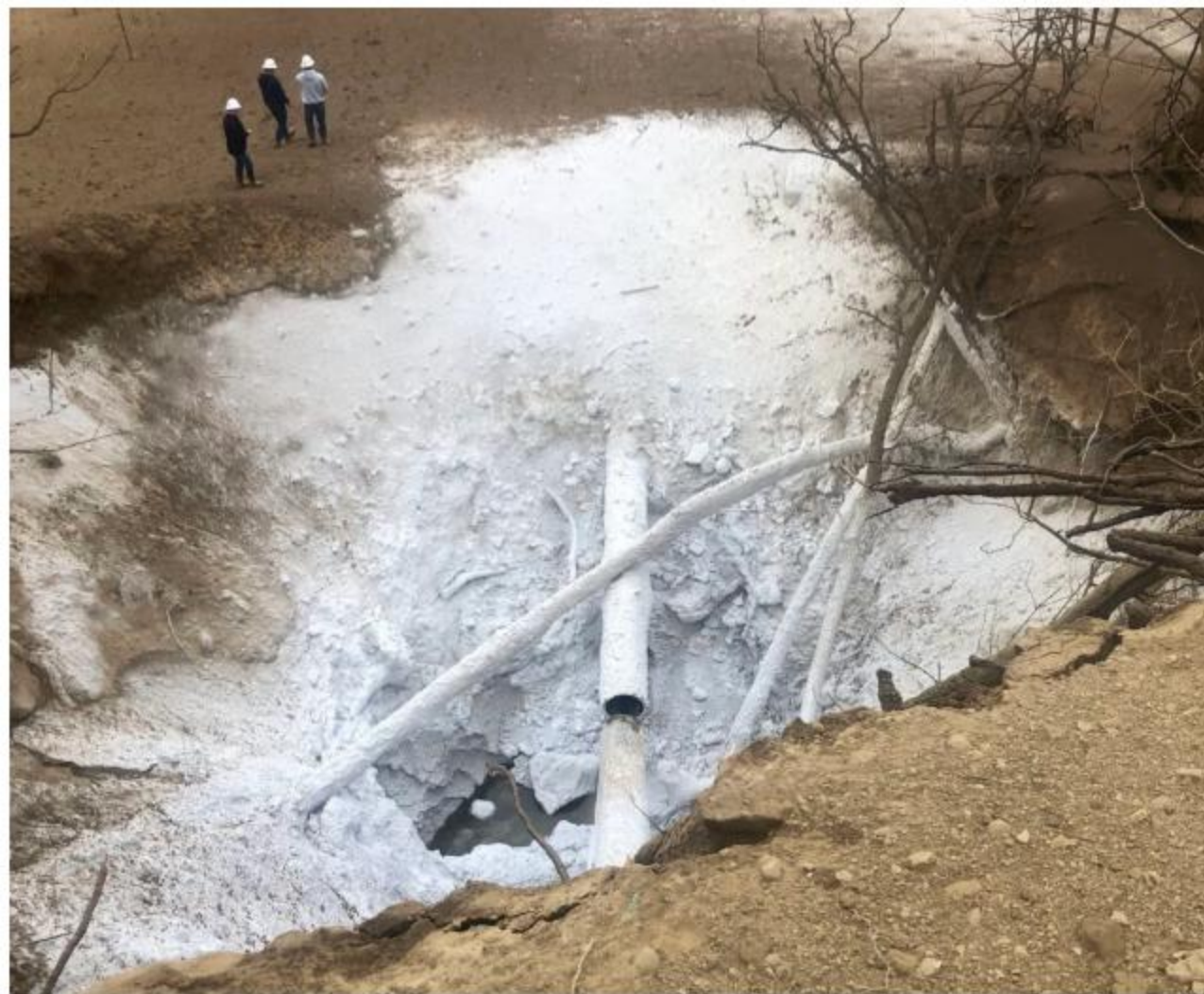
A CO 2 pipeline rupture in Yazoo County Mississippi in February 2020. (Yazoo County Emergency Management Agency)
